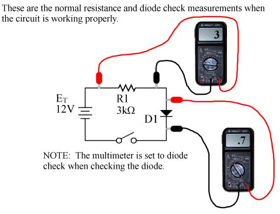
These are the normal resistance and diode check measurements when the circuit is working properly.  $E_{T} = R_{1}$  $R_{1}$  $R_{1}$  $R_{1}$  $R_{1}$  $R_{2}$  $R_{3}$  $R_{1}$  $R_{1}$  $R_{1}$  $R_{1}$  $R_{2}$  $R_{3}$  $R_{1}$  $R_{1}$  $R_{1}$  $R_{1}$  $R_{2}$  $R_{3}$  $R_{1}$  $R_{1}$  $R_{1}$  $R_{1}$  $R_{2}$  $R_{1}$  $R_{1}$  $R_{1}$  $R_{1}$  $R_{1}$  $R_{2}$  $R_{1}$  $R_{2}$  $R_{1}$  $R_{1}$
