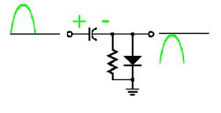
The negative alternation of the input signal reverse biases the diode.
