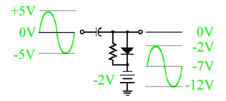
Remember, a biased clamper works just like an unbiased clamper.
