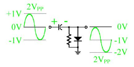
Select the correct output for this diode clamper.
