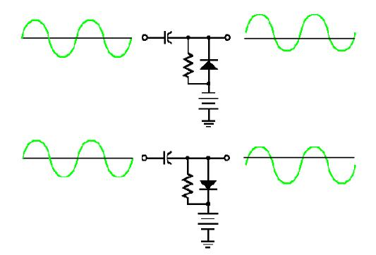
A positive bias on a positive clamper raises the output voltage DC level.
