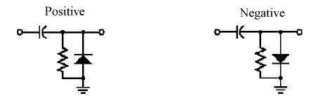
A positive clamper has the diode pointing up. The output signal will move in the direction the diode is pointing.
