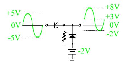
A positive bias on a negative clamper raises the output voltage DC level.
