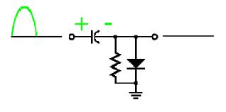
Adding the negative voltage stored in the capacitor to the positive peak voltage of the input signal produces a half cycle in the negative region with 0 volts at the outputs highest point.
