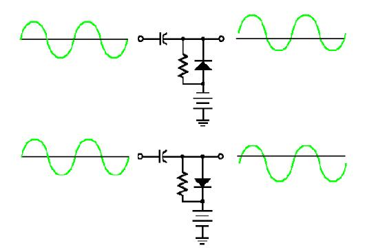
A clamper's effect on an input signal depends on how circuit components are connected.
