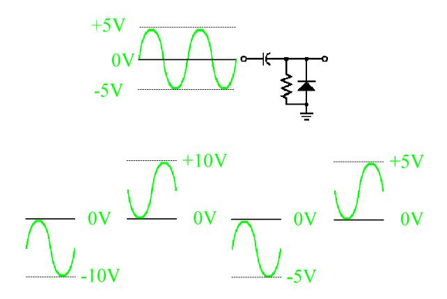
Select the correct output for this diode clamper.
