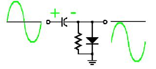
The peak to peak value of the output signal does not change, only the DC level.
