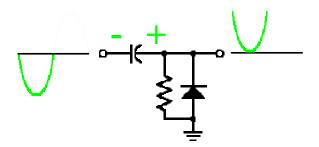
The positive alternation of the input signal reverse biases the diode.
