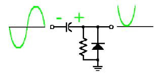
Adding the positive peak voltage of the input signal to the positive voltage stored in the capacitor doubles the output voltage.
