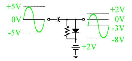
A negative bias on a negative clamper lowers the output voltage DC level.
