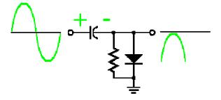
Adding the negative peak voltage of the input signal to the negative voltage stored in the capacitor doubles the output voltage.
