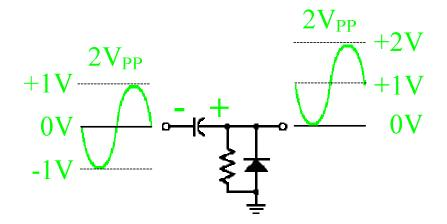
A negative clamper has the diode pointing down. The output signal will move in the direction the diode is pointing.
