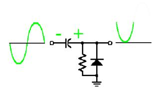
The peak to peak value of the output signal does not change, only the DC level.
