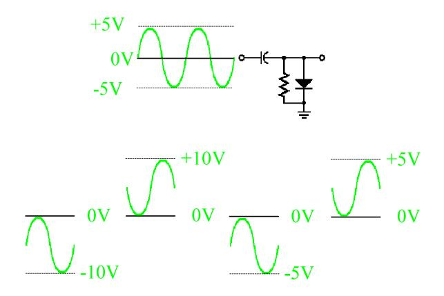
By adding circuit bias, the voltage level of the peaks are changed from 0 volts.
