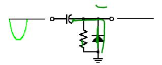
The capacitor quickly charges to the peak value with the positive polarity on the output.
