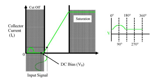
An advantage of class C operation is that it the highest efficient. Collector current  $(I_c)$  flows for less than 180 ° of the input signal.
