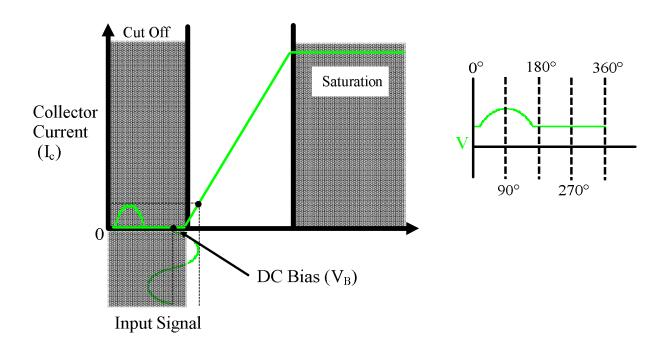
Class C amplifiers are normally used in RF turned amplifier applications. Fidelity is not an issue in these applications.
