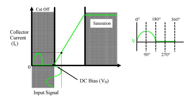
An advantage of class B operation is increased efficiency since the transistor is only conducting during half of the input signal.
