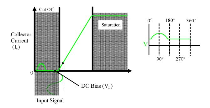
The transistor goes into saturation and cutoff if the amplitude of the input signal is too high. This is called overdriving the amplifier.
