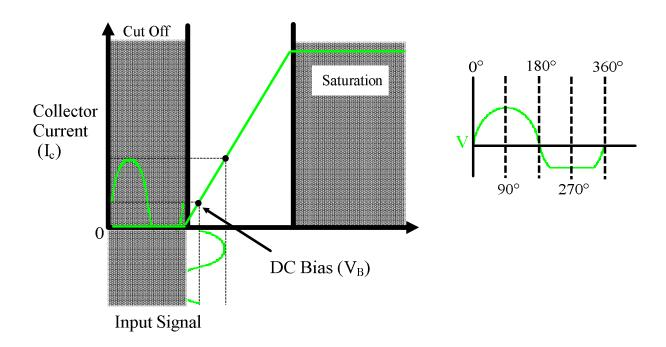
Class AB amplifiers are commonly used in place of class B push-pull amplifiers to overcome crossover distortion.
