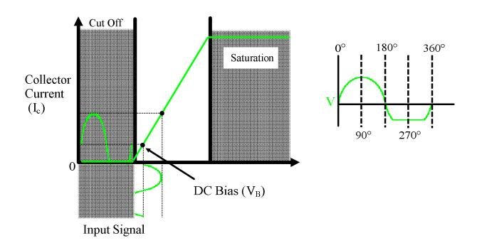
Class C amplifiers are biased so that collector current is zero for most of the input cycle.
