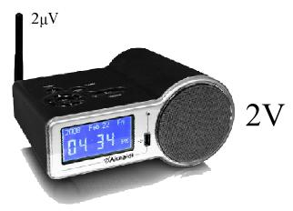
Amplifiers in the radio increase the voltage to about 2 volts. That is an increase of 1,000,000 times.
