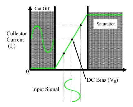
Class A amplifiers are biased so the input signal occurs within the limits of cutoff and saturation.
