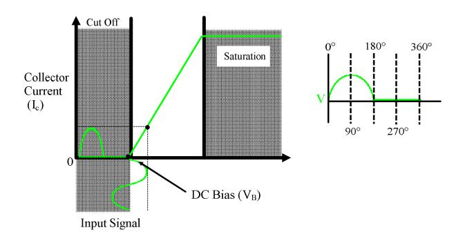
Class AB amplifiers are biased so the collector current (I c) is zero for a portion of one alternation.
