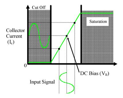
The point where a transistor is DC biased determines the class of operation.
