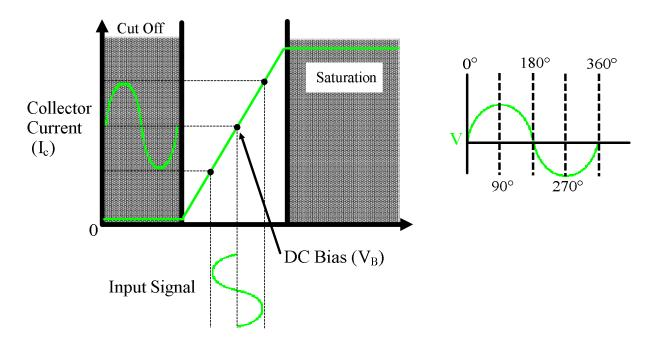
Class B amplifiers are biased so collector current is zero for half (one alternation) of the input signal.
