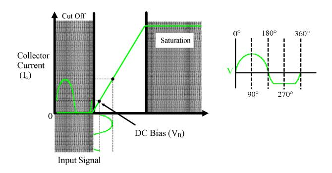
An advantage of class AB operation is that it is more efficient than class A and has better fidelity than class B.
