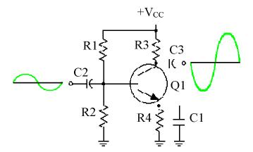
The coupling capacitors do not effect the bias voltages on Q1.
