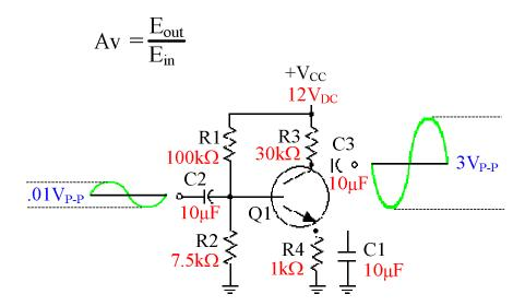
However, if the input and output signal voltage are unknown, gain can be calculated using the component values and the following formula.
