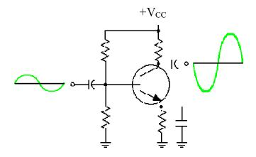
Transistor bias is determined by R1, R2, R3, R4, and C1.
