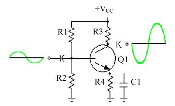
The result is a signal on the output that is a replica of the input signal except it is amplified and inverted.
