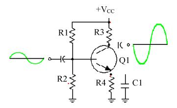
Any change in the fixed bias of Q1 produces a predicted change at the output.
