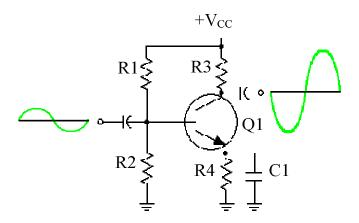
R4 provides temperature stability by decreasing emitter current when current increases due to heat.
