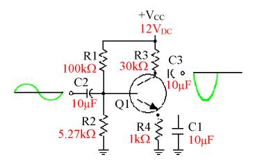
The actual component values determine the class of operation and voltage gain.
