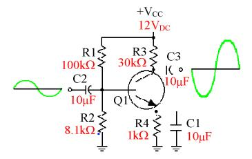
If the transistor is cutoff at any point on the input signal and the base voltage is greater than .6 volts, the class of operation is AB.
