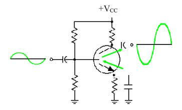
Note, an increasing input signal produces a decreasing output signal.
