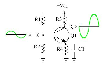
The output signal is determined by collector load resistor R3.
