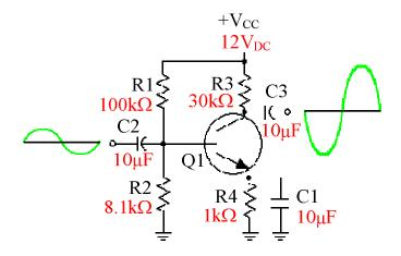
If class of operation and voltage gain are unknown, normal operation is determined by comparing input and output signals.
