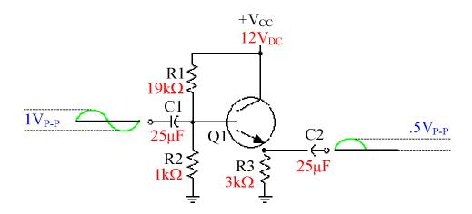
Determine class of operation for this common emitter circuit.
