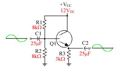
If the transistor is cutoff at any point on the input signal, the class of operation is AB.
