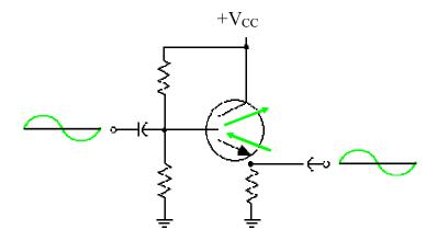
Note, an increasing input signal produces an increasing output signal. A decreasing input signal produces a decreasing output signal. The input signal controls the output signal.
