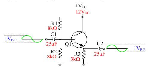
It is important to remember that common collector amplifiers produce a large current gain even through the voltage gain is 1.
