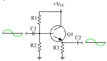
The coupling capacitors do not effect the bias voltages on Q1.
