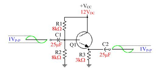
An input voltage of  $1V_{P-P}$  changes the base voltage from 6 volts to a range of 6.5V to 5.5V.
