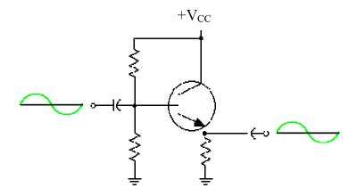
Transistor bias is determined by R1, R2, and R3.
