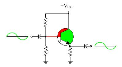
Notice the collector is common in both parts.
