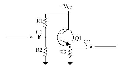
Any change in the fixed bias of Q1 produces a predicted change at the output. The collector is biased by +V  $_{\rm CC}$
