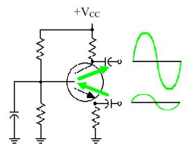
Note, an increasing input signal produces an increasing output signal.
