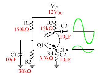
If class of operation and voltage gain are known, comparison of input and output signals determine if the amplifier is operating normally.
