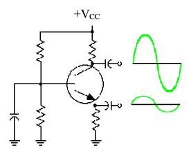
Transistor bias is determined by R1, R2, R3, R4, and C1.
