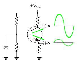
When the input signal decreases, the voltage on the emitter decreases, increasing forward bias on the base-to-emitter PN junction.
