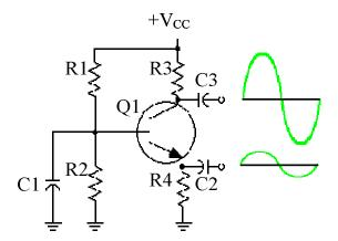
The coupling capacitors do not effect the bias voltages on Q1.
