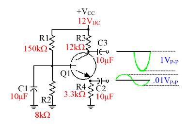
If the base bias on Q1 is less than .6 V, the class of operation becomes class C. The output signal shows less than  $180^{\circ}$ .
