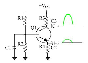
A decreasing input signal increases current. More voltage drops across R3 and the output signal decreases.
