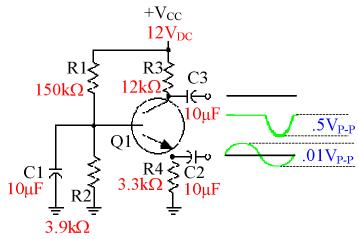
This is a class A common base with a gain of 200. The input to output comparison shows normal operation.
