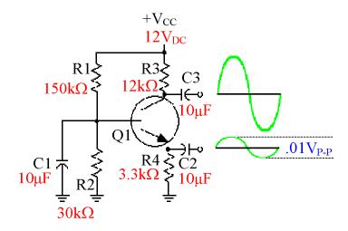
Find the class of operation by calculating the base voltage. It must be above .6 volts and the input signal cannot place the transistor into cutoff for class A.
