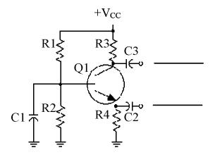
Resistor R4 establishes emitter bias. Any change in the emitter voltage produces a predictable change at the output.
