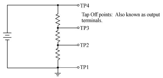
Ground is the zero reference point of a circuit.
