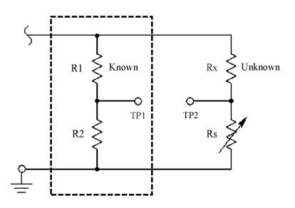
The voltage divider of Rx and Rs are unkown.
