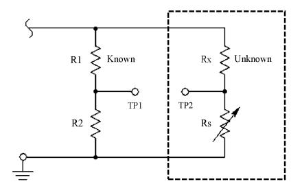
The voltage between TP1 and TP2 are compared for differences.
