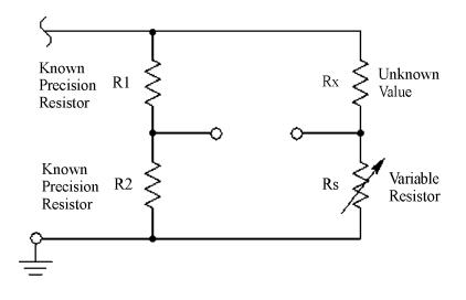
The voltage divider of R1 and R2 are a reference.
