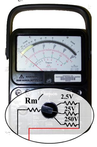
When measuring current, a multimeter is in series with the circuit.
