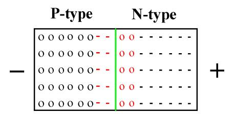
If the voltage potential is reversed, the depletion region at the PN junction would increase.
