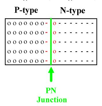
The PN junction is from the combination of free electrons and holes between the the P-type and N-type material.
