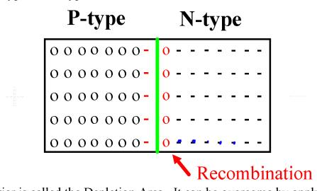
This barrier is called the Depletion Area. It can be overcome by applying a DC voltage (called **bias**) to the diode.
