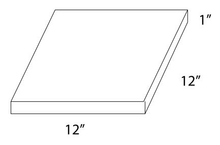
The volume of one board foot is calculated as:  $12^{\circ} \times 12^{\circ} \times 1^{\circ} = 144$  inches<sup>3</sup>
