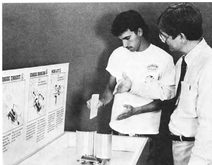
Fig. 3. When the deflector plates are used on the fan cart, airplane engine braking can be demonstrated.
